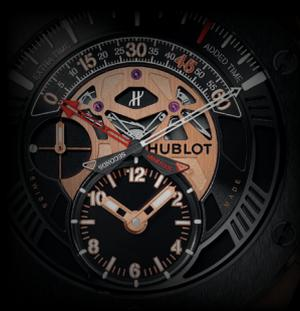
When the chronograph is started, the chrono's second hand and minute hand move from left to right in a circular arc of 45 minutes (one half of a football match). The watch also indicates an area for 15 minutes' «added time» up to 60 minutes and a second area for 15 minutes' «extra time».
