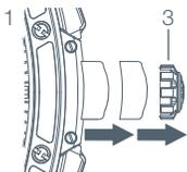
This function enables you to set the date displayed by the watch rapidly, without changing the time, using only the crown.
