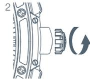
**Do not forget to screw the crown back in completely to ensure its water resistance.**
